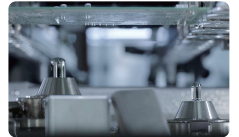
双缸独立电磁泵选择性波峰 Double-cylinder independent electromagnetic pump selective crest
